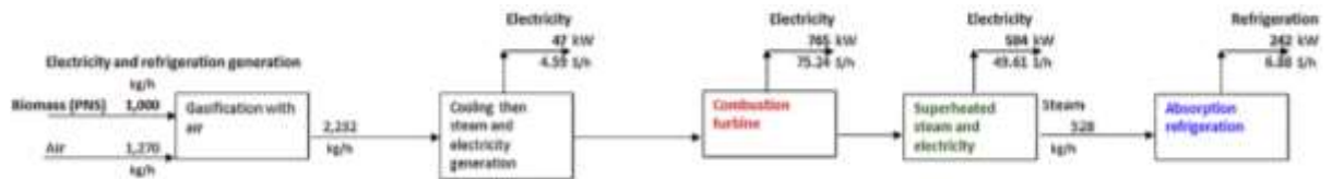
Fig. 2.2. Electricity and refrigeration processes
