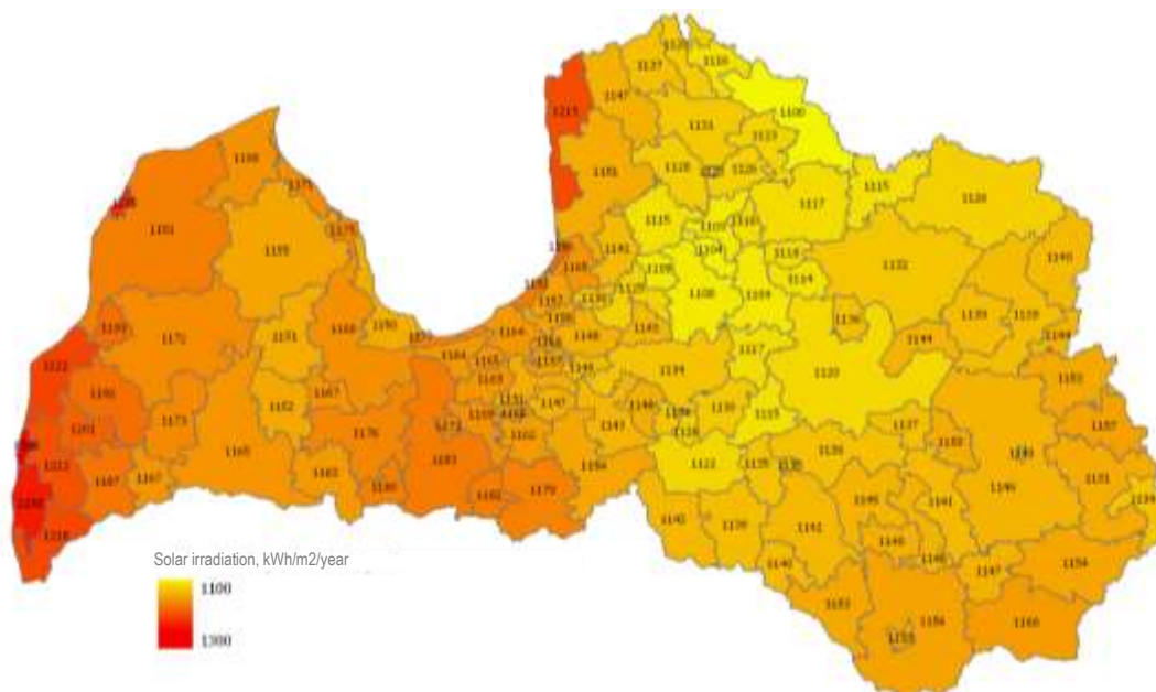
Fig. 1.25. Solar irradiation in municipalities, kWh/m 2 /year (GIS layout, data source: Photovoltaic Geographical Information System)
